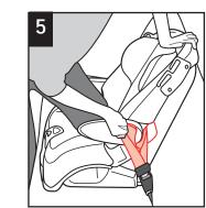
Place one knee in the child restraint and push down firmly while pulling up on the loop to tighten belt.
